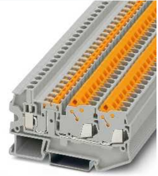
2.5 (2.5) mm 2 , 20 A, knife disconnect terminal block, three connections
