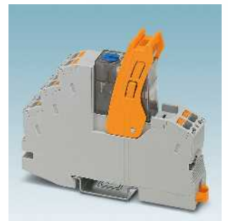
Relay modules - RIFLINE complete - Fully mounted RIF-1 relay modules with relay with detectable manual operation, status LED, and push-in connection
