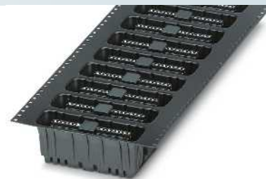
Pin length of 2.0 mm, taped PCB terminal blocks, connection direction vertical to the PCB
