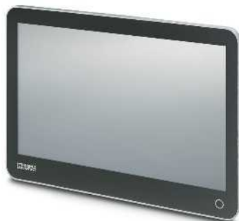
Fully enclosed IP65 IPC with 54.6 cm (21.5") display
