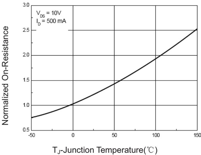
**Figure 9 Drain-Source On-Resistance**
