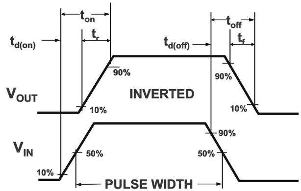
**Figure 2: Switching Waveforms**
