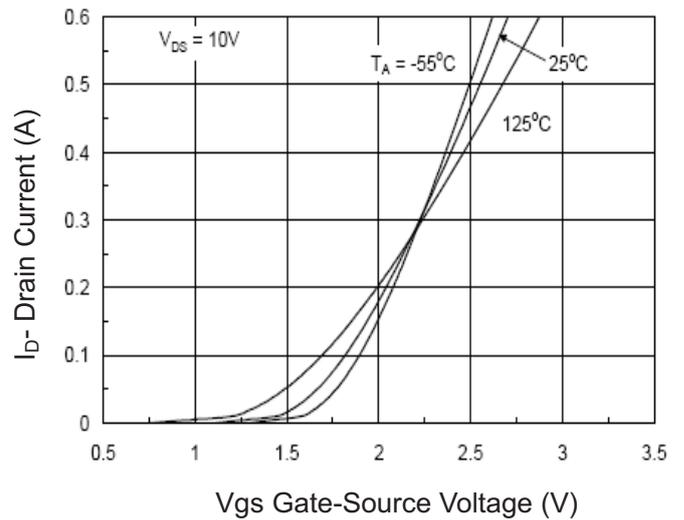
**Figure 4 Transfer Characteristics**
