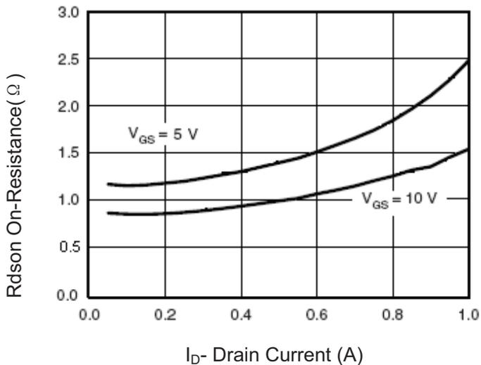
**Figure 5 Drain-Source On-Resistance**
