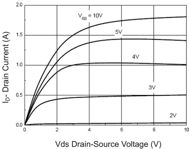
**Figure 3 Output Characteristics**
