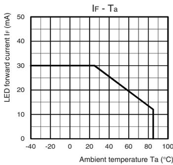
Continuous load current vs. Ambient temperature
