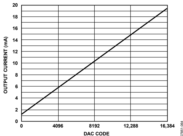
Figure 63. Gain Curve for FSC[9:0] = 512, DAC Offset = 1.228 mA
