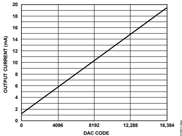
Figure 63. Gain Curve for FSC[9:0] = 512, DAC Offset = 1.228 mA
