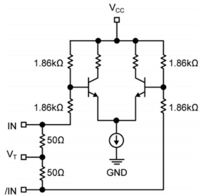
Figure 3a. Simplified Differential Input Stage
