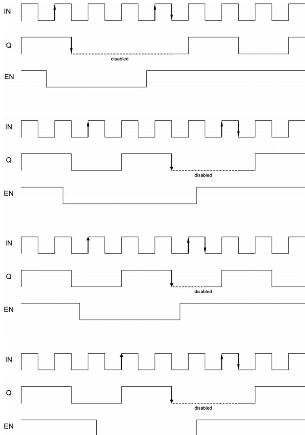
Figure 1c. Enable Output Timing Diagram Examples (divide by 3)
