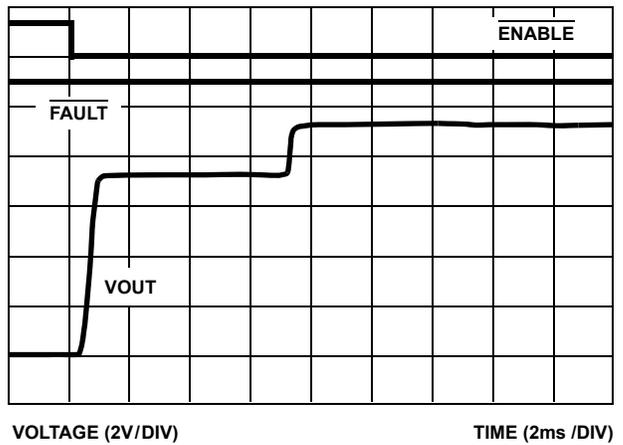
FIGURE 11. ISL6119L TURN-ON INTO 1.5A MOMENTARY OC
