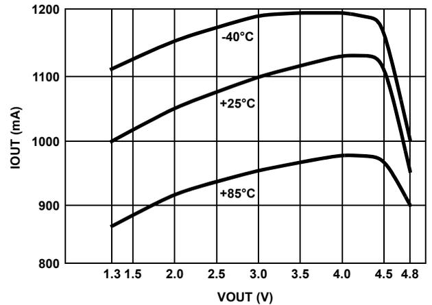
FIGURE 5. CURRENT REGULATION vs VOUT (VIN = 5.0V)
