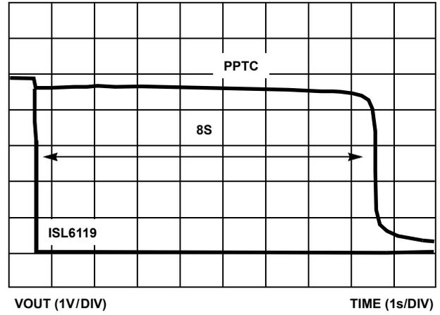
FIGURE 15. ISL6119 vs PPTC WITH EXTENDED 1.5A LOAD
