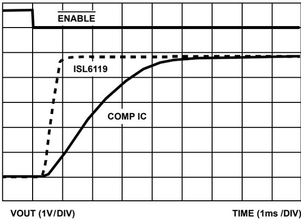
FIGURE 16. COMPARATIVE TURN-ON WAVEFORMS, RI = 10Ω
