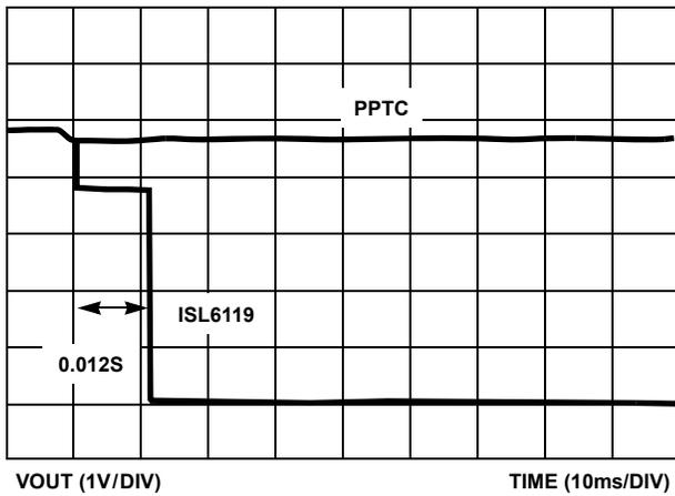
FIGURE 14. ISL6119 vs PPTC PLUGGED ONTO 1.5A LOAD
