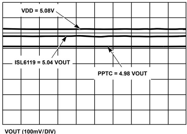
FIGURE 13. ISL6119 vs PPTC INTO 500mA LOAD
