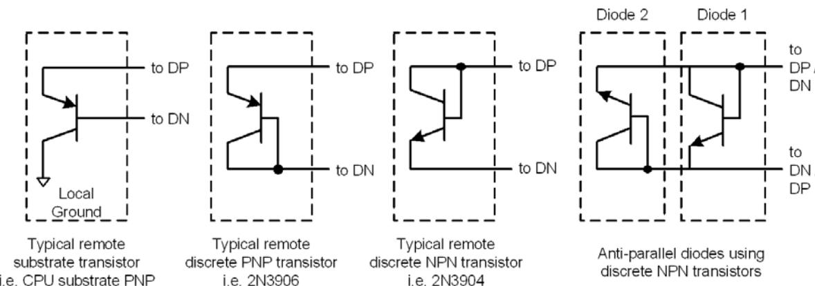
Figure 5.7 Diode Connections
