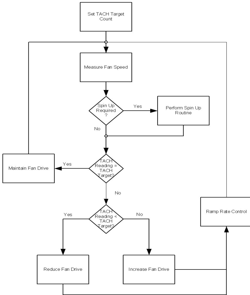
Figure 5.4 RPM based Fan Speed Control Algorithm
