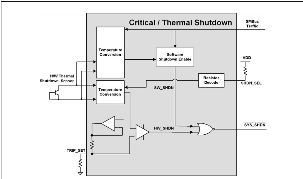
Figure 5.2 Block Diagram of Critical / Thermal Shutdown
