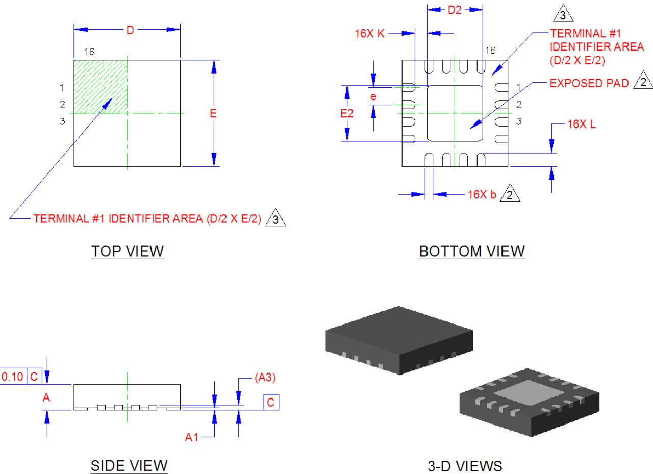
Figure 7.5 16-Pin QFN 4mm x 4mm Package Drawing
