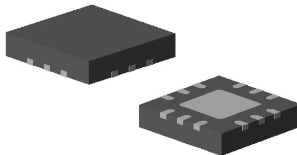
**3-D VIEWS****Figure 7.2 12-Pin QFN 4mm x 4mm Package Drawing**
