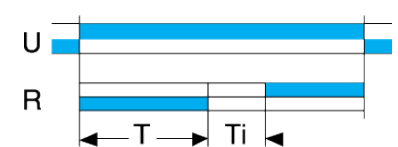
Function Q: “Star-delta” starting
