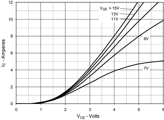
**Fig. 2. Extended Output Characteristics @  $T_J = 25^\circ\text{C}$**
