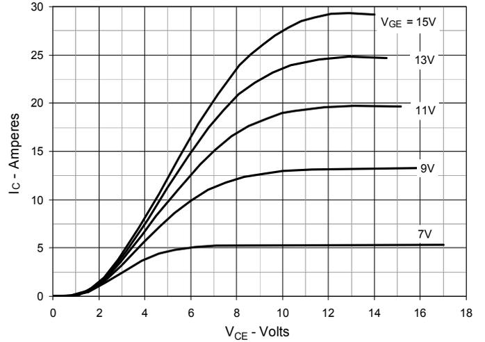
**Fig. 3. Output Characteristics @  $T_J = 125^\circ\text{C}$**
