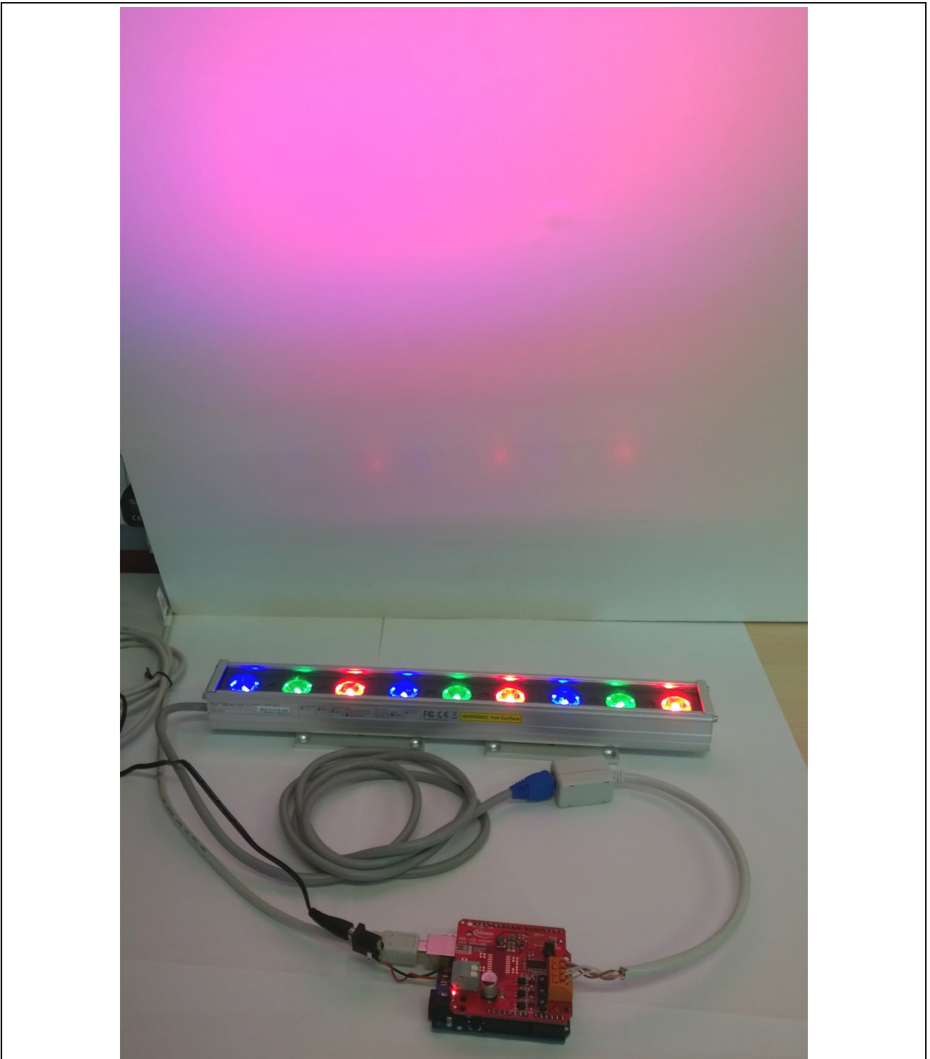
RGB LED Shield driving an LED wall washer
