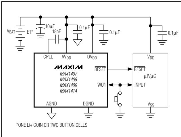
Figure 22. Power-Supply Circuit Using Direct Battery Connection
