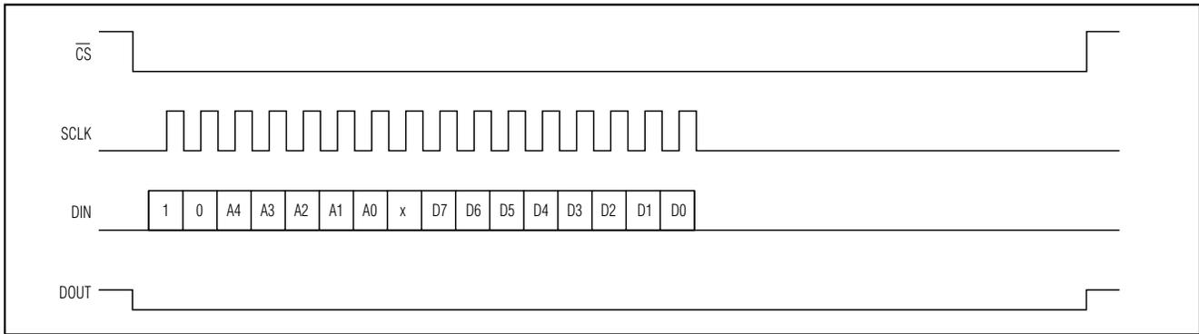
Figure 12. Serial Interface 8-Bit Write Timing Diagram
