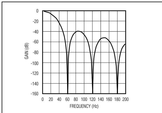
Figure 7. Frequency Response of the SINC<sup>3</sup> Filter (Notch at 60Hz)
