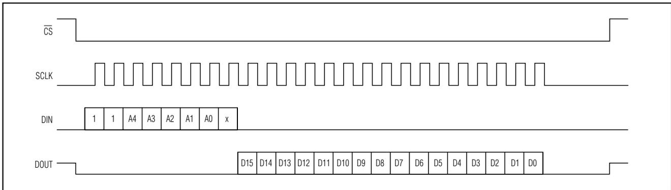
Figure 13. Serial Interface 16-Bit Read Timing Diagram
