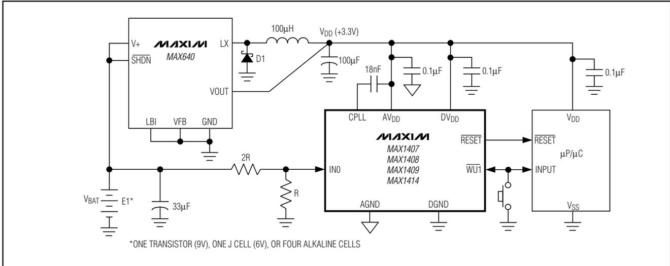
Figure 21. Power-Supply Circuit Using MAX640 Step-Down DC-DC Converter
