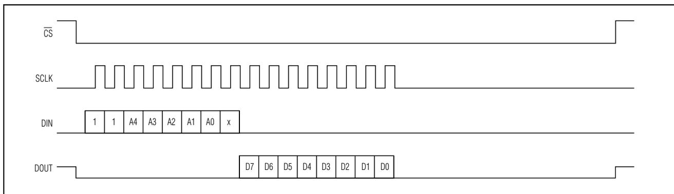
Figure 14. Serial Interface 8-Bit Read Timing Diagram
