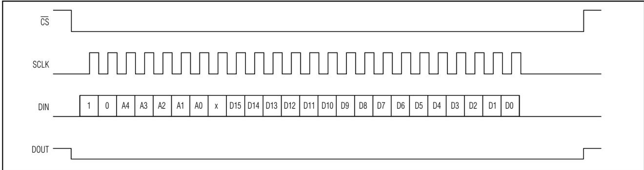
Figure 11. Serial Interface 16-Bit Write Timing Diagram
