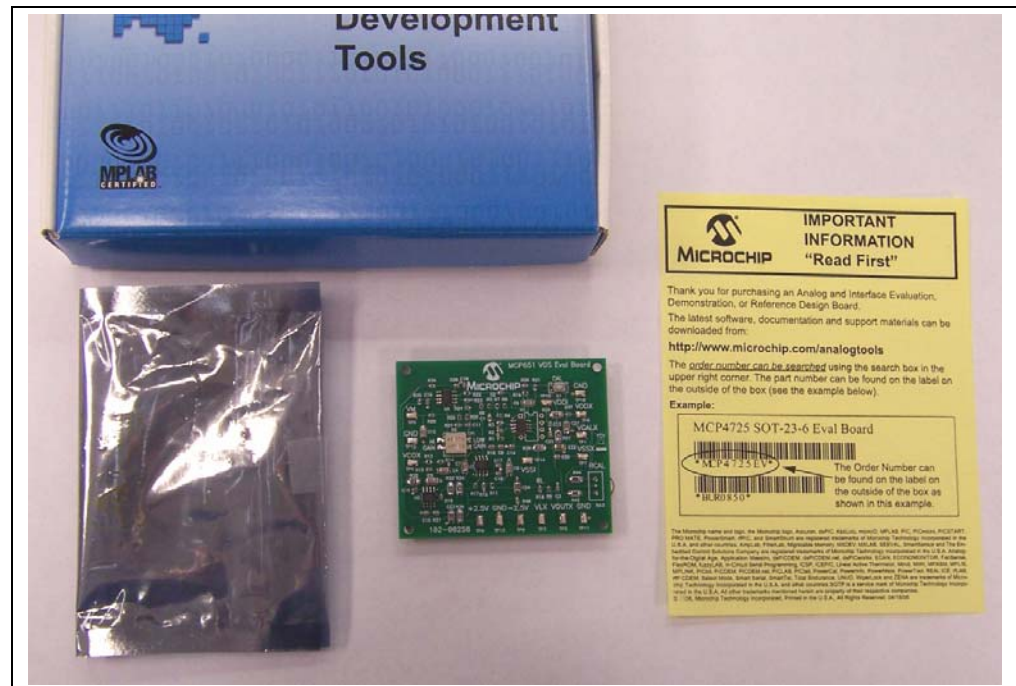
FIGURE 1-1: MCP651 Input Offset Evaluation Board Kit Contents.
