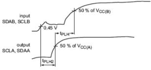
Figure 14. Propagation Delay
