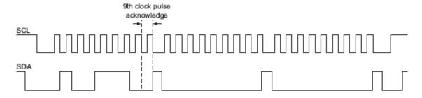
Figure 4. Bus A (0.9 V to 5.5 V Bus) Waveform
