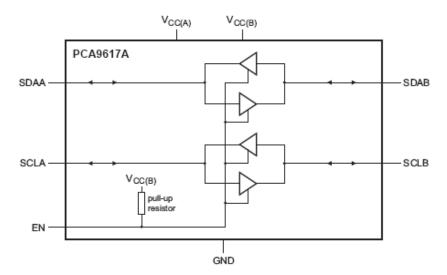
Figure 1. Block Diagram of PCA9617A
