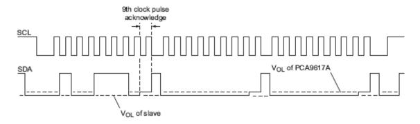
Figure 5. Bus A (0.9 V to 5.5 V Bus) Waveform
