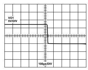
FIGURE 5. SHUTDOWN USING I<sup>2</sup>C ENABLE
