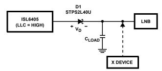
FIGURE 11. DC BACK-BIAS PROTECTION CIRCUIT
