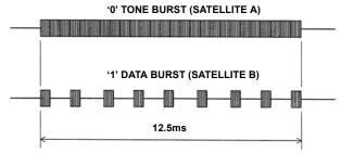
FIGURE 2. TIMING DIAGRAM FOR TONE BURST CONTROL SIGNAL
