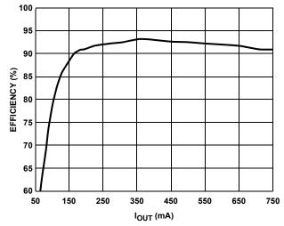
FIGURE 6. BOOST PWM EFFICIENCY vs LOAD
