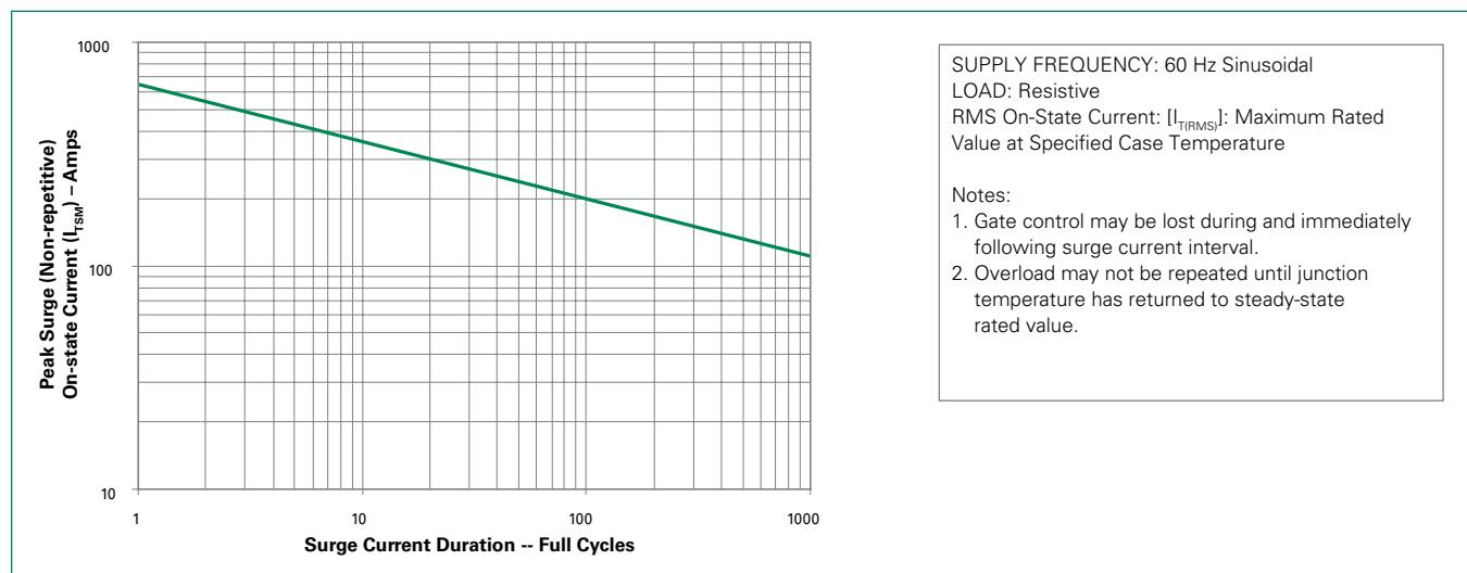
SUPPLY FREQUENCY: 60 Hz Sinusoidal
