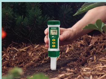
**Rugged waterproof (IP57) housing with Flat Surface Electrode for measuring pH in liquids, semi-solids, and solids. Does not break or get junctions clogged like traditional glass bulb electrodes. Easy to replace sensor is perfect for field or lab use.**
