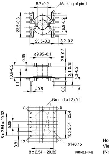
Hole arrangement View in mounting direction (Note half pitch!)
