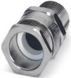
Cable gland, Cable gland material: Nickel-plated brass, Application: Ex, External cable diameter 11.1 mm ... 20 mm, Shielding: No, Connecting thread: M25, Color: silver
