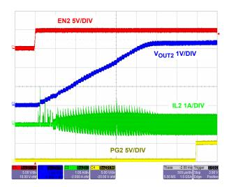
FIGURE 26. START-UP  $V_{OUT2} = 3.3V$  (NO LOAD)
