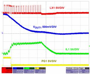
FIGURE 31. V<sub>OUT1</sub> = 1.2V OUTPUT OVERCURRENT
