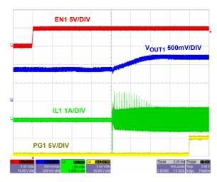
FIGURE 23. START-UP V<sub>OUT1</sub> = 1.2V (UNDER PRE-BIASED)
