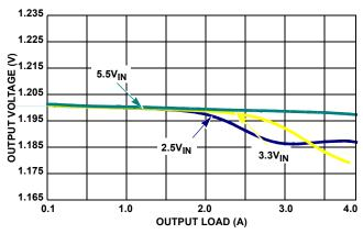
FIGURE 10. V<sub>OUT1</sub> = 1.2V REGULATION vs LOAD
