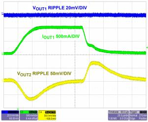
FIGURE 30. V<sub>OUT1</sub> = 1.2V LOAD TRANSIENT
