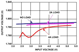
FIGURE 15.  $V_{OUT1}$  = 1.8V REGULATION vs  $V_{IN}$
