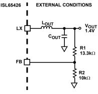
FIGURE 36. EXTERNAL OUTPUT VOLTAGE SELECTION
