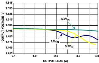
FIGURE 12. V<sub>OUT1</sub> = 1.5V REGULATION vs LOAD
