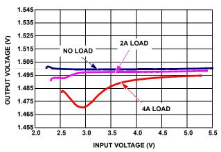
FIGURE 13.  $V_{OUT1}$  = 1.5V REGULATION vs  $V_{IN}$
