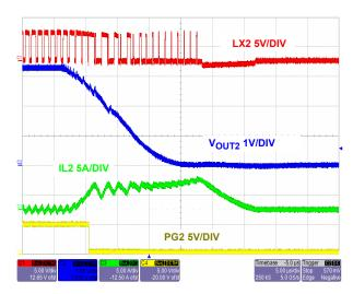
FIGURE 33. V<sub>OUT2</sub> = 3.3V OUTPUT OVERCURRENT
