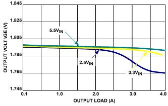
FIGURE 14. V<sub>OUT1</sub> = 1.8V REGULATION vs LOAD
