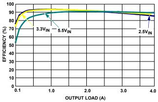
FIGURE 5. V<sub>OUT1</sub> = 1.5V EFFICIENCY vs LOAD
