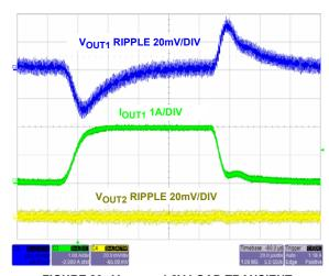
FIGURE 29. V<sub>OUT1</sub> = 1.2V LOAD TRANSIENT
