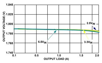
FIGURE 16. V<sub>OUT2</sub> = 1.8V REGULATION vs LOAD
