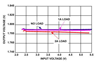
FIGURE 17. V<sub>OUT2</sub> = 1.8V REGULATION vs VIN
