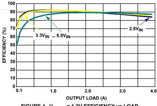
FIGURE 4. V<sub>OUT1</sub> = 1.2V EFFICIENCY vs LOAD
