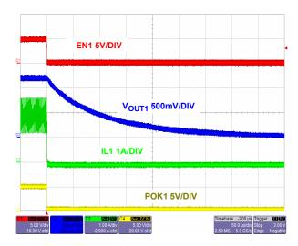
FIGURE 25. SHUTDOWN V<sub>OUT1</sub> = 1.2V
