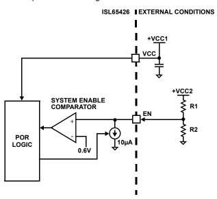
FIGURE 37. SYSTEM ENABLE INPUT
