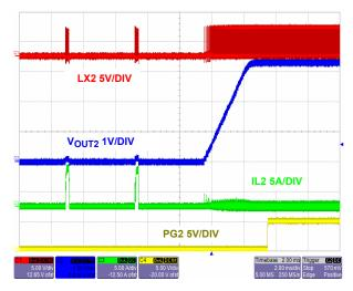
FIGURE 34. V<sub>OUT2</sub> = 3.3V OUTPUT OVERCURRENT RECOVERY
