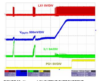
FIGURE 32. V<sub>OUT1</sub> = 1.2V OUTPUT OVERCURRENT RECOVERY
