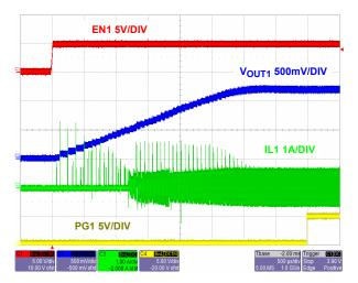
FIGURE 22. START-UP V<sub>OUT1</sub> = 1.2V (NO LOAD)
