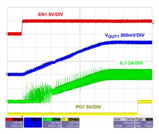
FIGURE 24. START-UP V<sub>OUT1</sub> = 1.2V (FULL LOAD)
