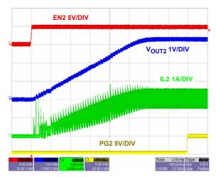
FIGURE 28. START-UP  $V_{OUT2} = 3.3V$  (FULL-LOAD)
