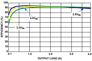
FIGURE 6. V<sub>OUT1</sub> = 1.8V EFFICIENCY vs LOAD
