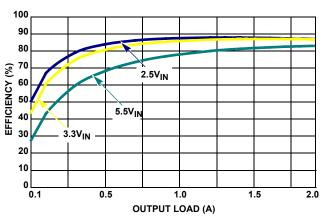
FIGURE 7. V<sub>OUT2</sub> = 1.8V EFFICIENCY vs LOAD
