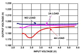
FIGURE 11. V<sub>OUT1</sub> = 1.2V REGULATION vs V<sub>IN</sub>
