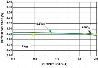
FIGURE 20. V<sub>OUT2</sub> = 3.3V REGULATION vs LOAD
