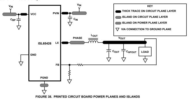
Sensitive signals should be routed on different layers or some distance away from the PHASE plane on the same layer. Crosstalk due to switching noise is reduced into these lines by isolating the routing path away from the PHASE plane. Layout the PHASE planes on one layer, usually the top or bottom layer, and route the voltage feedback traces on another remaining layer.
