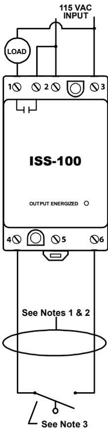
1. Maximum distance between unit and switch contact is 10,000 feet.
