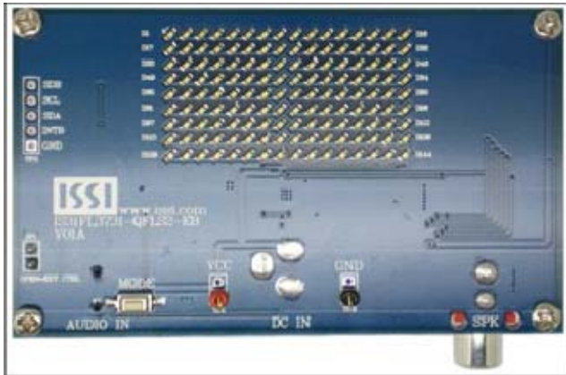
Figure 12: Photo of IS31FL3731 Evaluation Board
