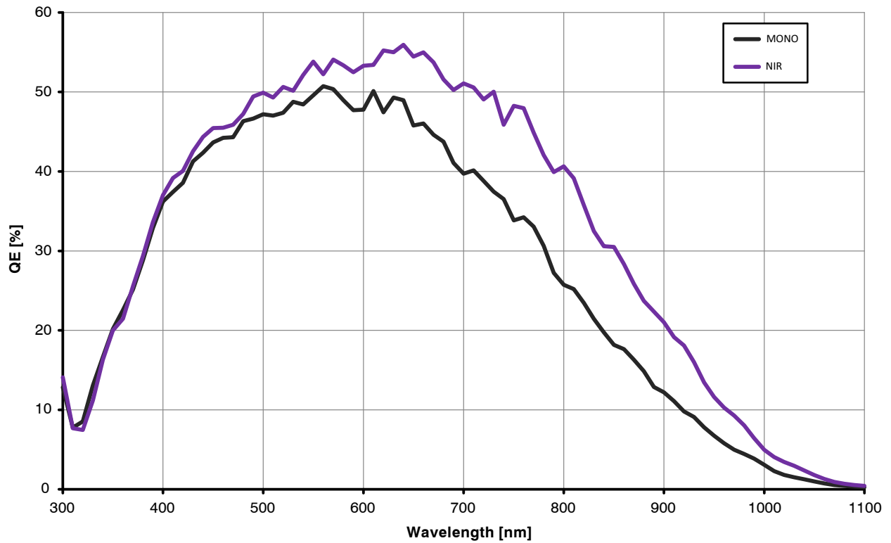
Figure 4. Quantum Efficiency Curve for Standard and NIR Mono
