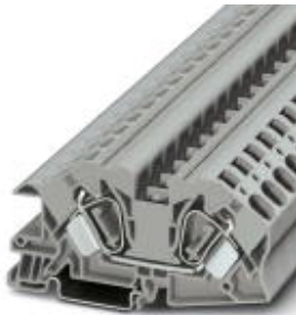
Installation level terminal block, Spring-cage connection, Cross section: 0.2 mm 2 - 25 mm 2 , AWG: 24 - 4, Width: 12 mm, Color: gray, Mounting type: NS 35/7,5, NS 35/15
