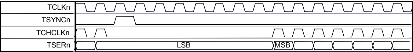
Figure 11-31. E1 Transmit-Side TCHCLKn Gapped Mode During Channel 1
