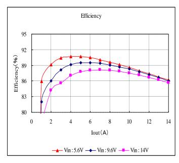
Fig. 12-3-8. Efficiency v.s. Output Current
