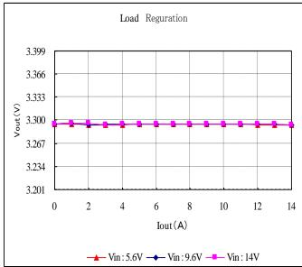
Fig. 12-3-1. Output Voltage v.s. Output Current
