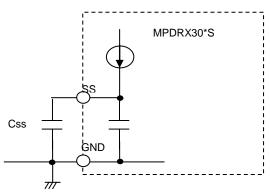
The equation of starting time about output voltage.
