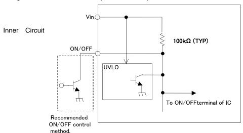
ON/OFF Control Operation When ON/OFF-pin(13pin) is left open When ON/OFF-pin(13pin) is connected to GND
