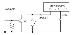
.. Output Voltage = ON.. Output Voltage = OFF
