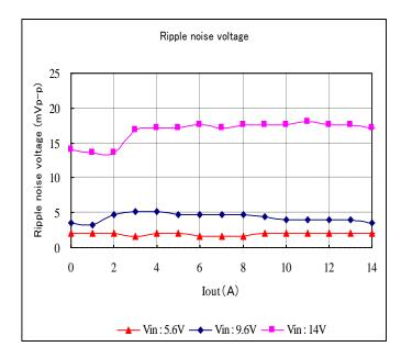
Fig. 12-3-9. Ripple Voltage v.s. Output Current
