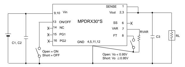
$\begin{array}{ll} \text{C1,C2}: 10\mu\text{F}\middle/25\text{V} & \text{(Ceramic Capacitor)} \\ \text{C3}: 100\mu\text{F}\middle/6.3\text{V} & \text{(Ceramic Capacitor)} \end{array}$
