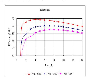
Fig. 12-3-2. Efficiency v.s. Output Current
