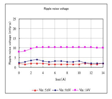
Fig. 12-3-15. Ripple Voltage v.s. Output Current
