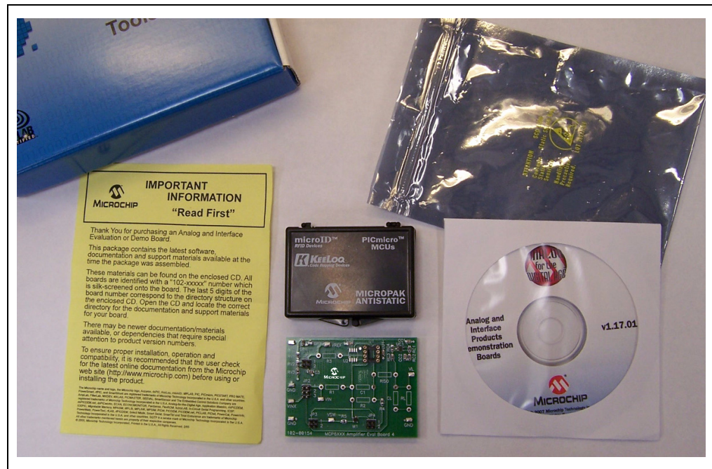
FIGURE 1-1: MCP6XXX Amplifier Evaluation Board 4 Kit.
