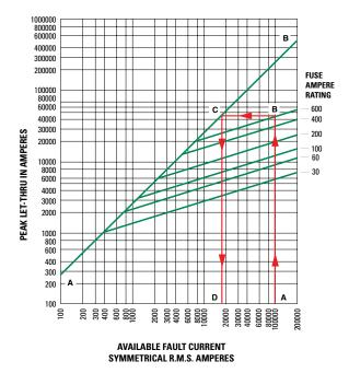
Figure 8 – Peak Let-through Chart for POWR-PRO® LLNRK Class RK1 Dual-Element Fuses Using the Up-Over-and-Down Method
