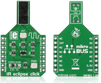
IR eclipse click™ carries an EE-SX198 photo interrupter sensor. This sensor consists of an infrared transmitter and receiver facing each other and spaced apart by a 3mm slit. When the beam from the transmitter is eclipsed with by placing an object in the gap (like a piece of paper), the sensor is activated (indicated by the onboard INT LED). IR eclipse click™ communicates with the target board through the mikroBUS™ INT line. It's designed to work with either a 3.3V or 5V power supply.
