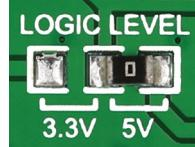
To switch between 3.3V or 5V power supplies, use the onboard zero-ohm SMD jumper. By default it's soldered in the 3.3V position.
