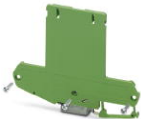
Side element with foot, tall design, left-hand, for 60 mm wide U-shaped cover, with PE contact to the DIN rail.
