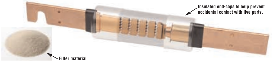
Figure 6. This is the LPS-RK100SP, a 100A, 600V LOW-PEAK®, Class RK1, Dual-Element Fuse that has excellent time-delay, excellent current-limiting and a 300,000A interrupting rating. Artistic liberty is taken to illustrate the internal portion of this fuse. The real fuse has a non-transparent tube and special small granular, arc-quenching material completely filling the internal space.
