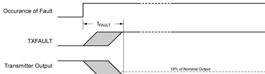
**Figure 18. Transmit Fault Timing**
