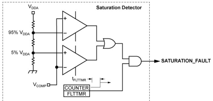
Figure 11. Saturation Detector
