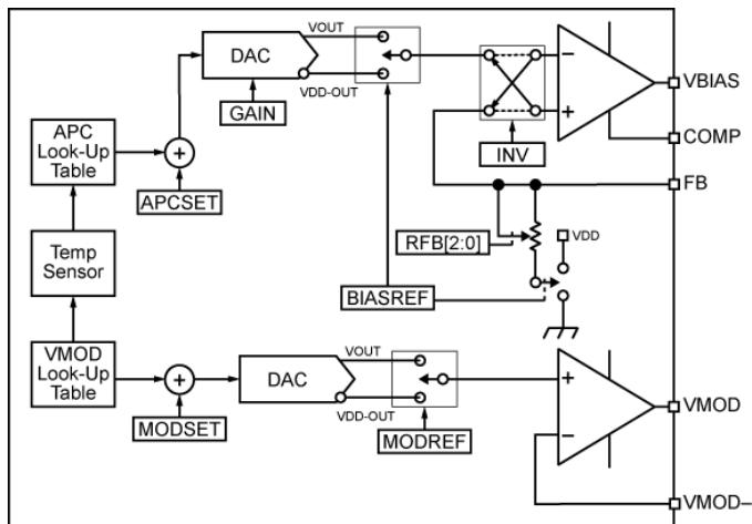
**Figure 5. APC and Modulation Control Block Diagram**
