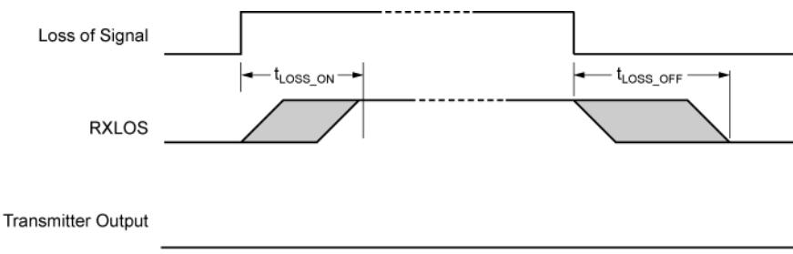
**Figure 17. Loss-of-Signal (LOS) Timing**
