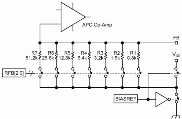
**Figure 6. Programmable Feedback Resistor**
