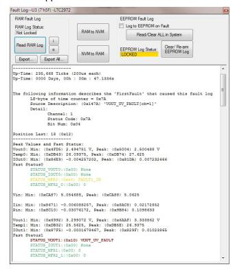
The log contains timestamp, up-time, channel voltage readings, an input voltage reading, an on-chip temperature reading, etc. There will be a number of loops; each loop contains data obtained in one ADC loop time with the most recent ADC loop data on top and the oldest data at the bottom of the log. The up-time indicates, at the time of fault, the amount of time the device had been powered up or time since the previous reset.
