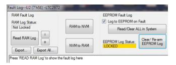
It is a 2-step process to read the fault log. First click the "NVM to RAM" button. At this point the RAM Log is locked. Click the "Read NVM Log" button. The fault log data will appear in the text box below.
