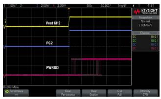
The scope shot shows  $V_{OUT}$  CH2, PG2, and PWRGD signals with infinite persistence. Multiple triggers show that PG asserts immediately and is predictable whereas PWRGD assertions are not only slower than PG but also the timing is variable.
