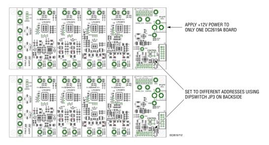
Figure 12. Array of Multiple Board Sets
