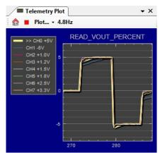
The LTC2972 has a multiplexed ADC that is used to provide voltage, current and temperature readback values. The telemetry plot in the GUI is similar to a multi-channel oscilloscope which is capable of displaying any parameter that is displayed in the telemetry window. Due to the nature of a multiplexed ADC converter, it has an associated ADC loop time of approximately 135ms.
