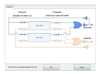
Figure 9. Fault Sharing Utility in LTpowerPlay GUI
