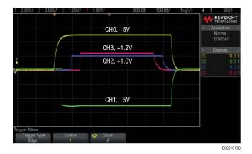
Figure 6. Sequencing Output Channels On/Off
