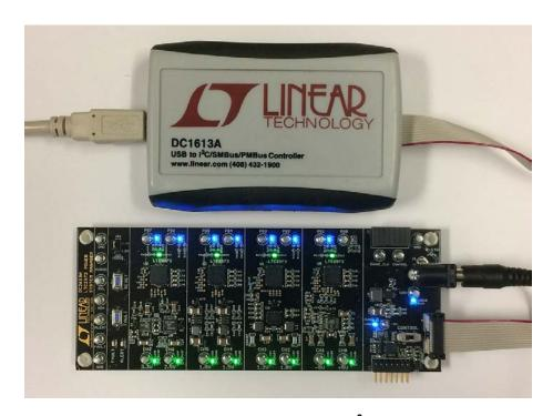
Figure 3. Connecting DC2619A and the DC1613 USB to I<sup>2</sup>C/SMBus/PMBus Controller
