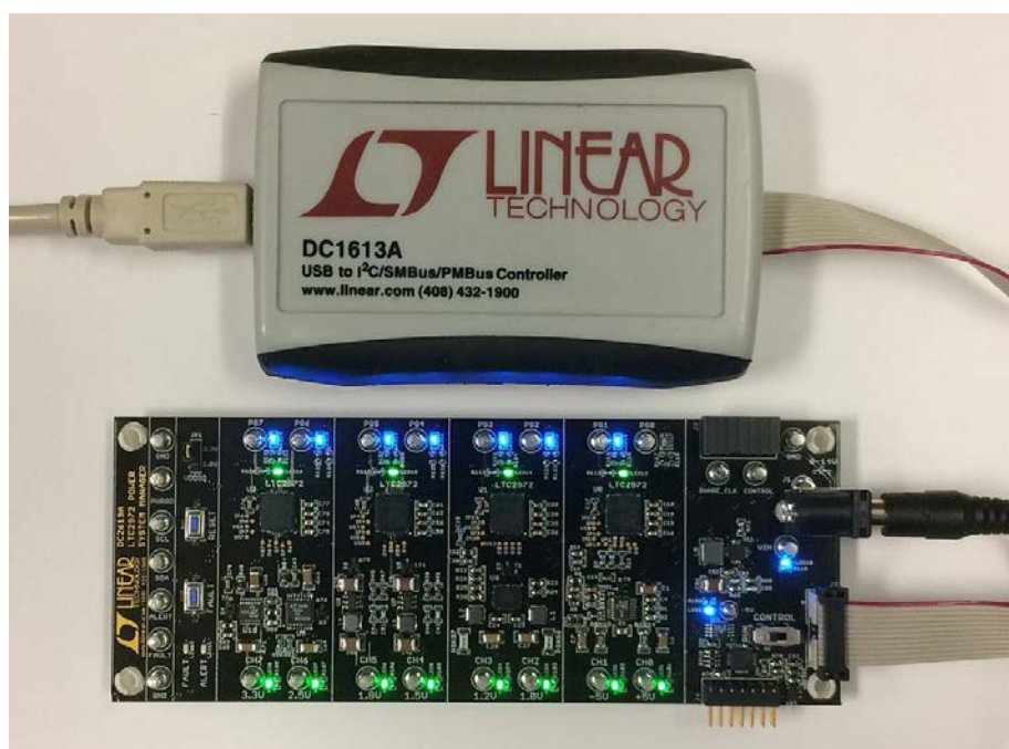
Figure 3. Connecting DC2619A and the DC1613 USB to I 2 C/SMBus/PMBus Controller
