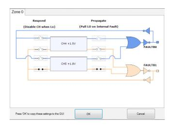
Figure 11. CH4 Fault Switches Open
