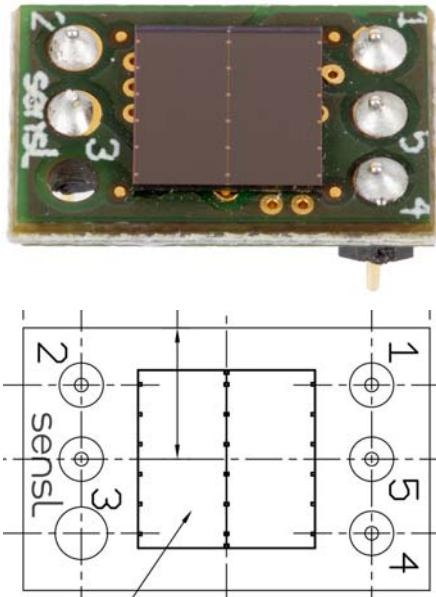
Figure 7. Top View of the SMTPA Board
