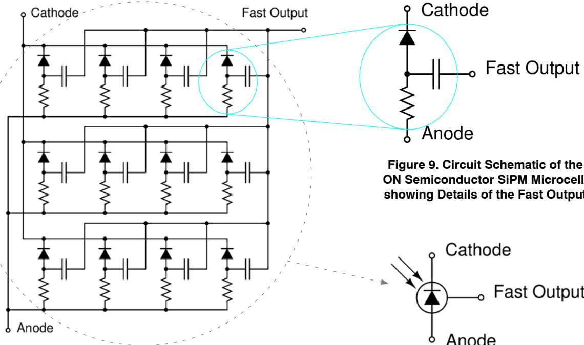
**Figure 10. Simplified Circuit Schematic of the ON Semiconductor SiPM showing only a 12 Microcell Example. Typically, SiPM Sensors have Hundreds or Thousands of Microcells**
