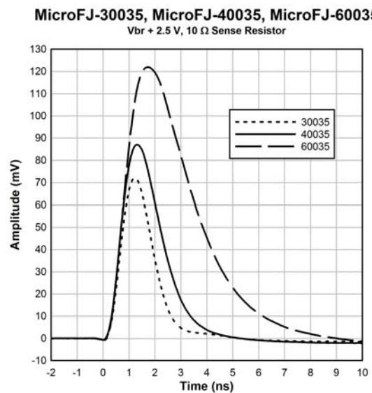
**Figure 5. Fast Output Pulse Shape**
