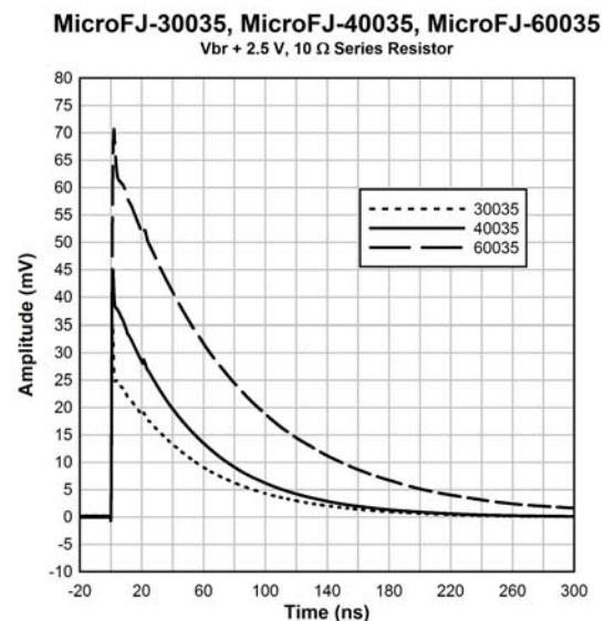
**Figure 6. Standard Output Pulse Shape**
