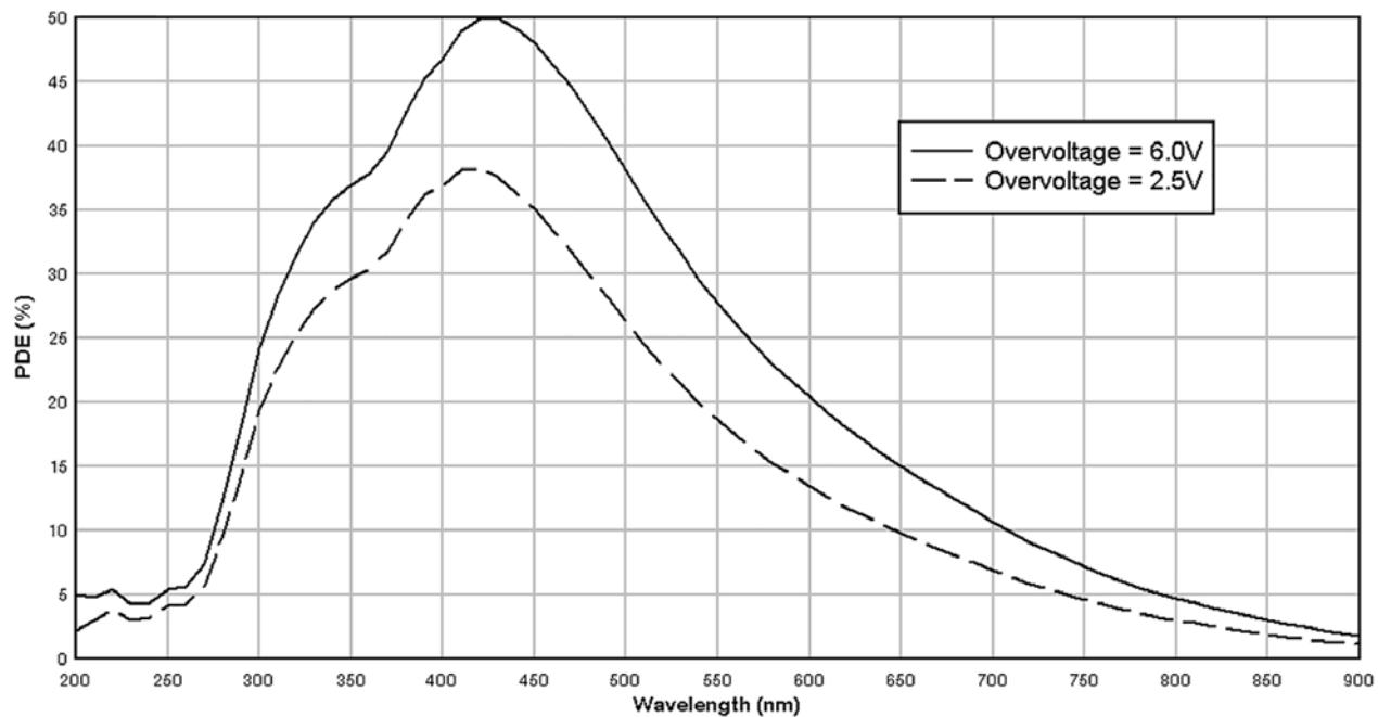
**Figure 1. Photon Detection Efficiency (PDE)**
