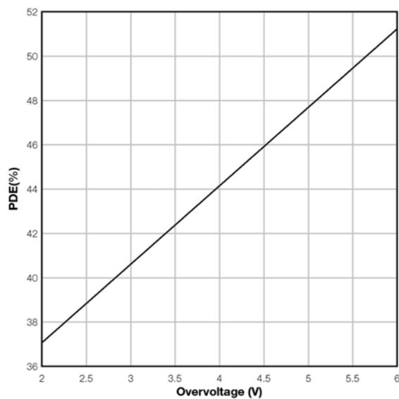
**Figure 2. PDE vs. Overvoltage**
