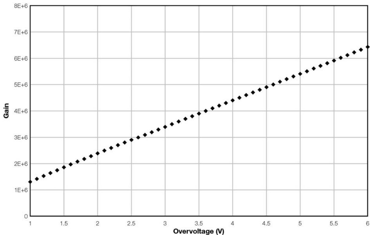
**Figure 4. Gain vs. Overvoltage**
