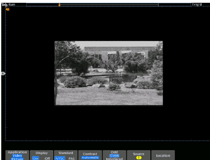
Viewing an NTSC video signal. Video picture mode contains automatic contrast and brightness settings as well as manual controls.
