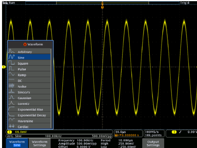
Waveform type selection in the integrated AFG.
