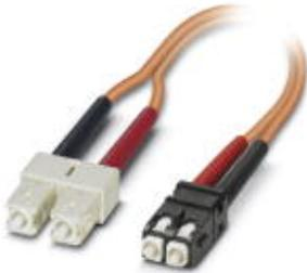
Assembled FO cable, zip cord cable, multi-mode fiberglass 50/125  $\mu\text{m}$ , OM2, plug: SC duplex/SCRJ, degree of protection: IP20, for installation in cable ducts or control cabinets, length: 2 m
