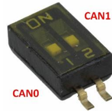
Figure 44: CAN Termination Switch
