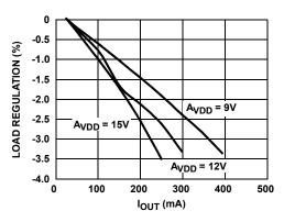
FIGURE 7.  $V_{BOOST}$  LOAD REGULATION AT  $V_{IN}$  = 3V (P-MODE)
