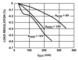
FIGURE 5.  $V_{BOOST}$  LOAD REGULATION AT  $V_{IN}$  = 3V (PI-MODE)
