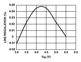
FIGURE 9. VBOOST LINE REGULATION (PI-MODE)
