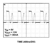
FIGURE 17. LX WAVEFORM - DISCONTINUOUS MODE
