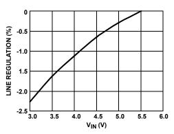
FIGURE 10. V<sub>BOOST</sub> LINE REGULATION (P-MODE)
