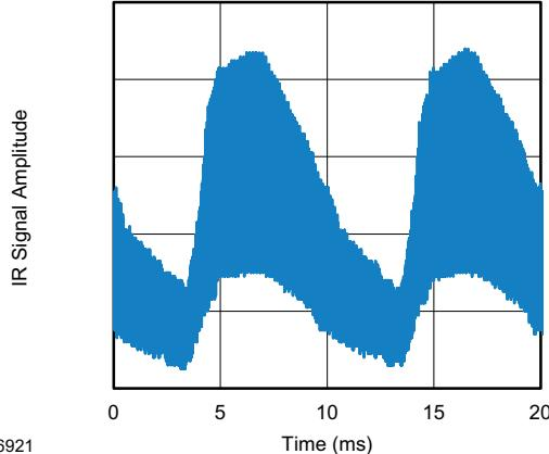
Fig. 14 - IR Emission from Fluorescent Lamp
