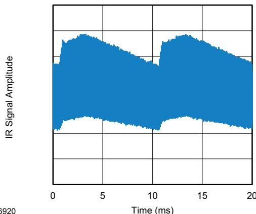
Fig. 13 - IR Emission from Fluorescent Lamp
