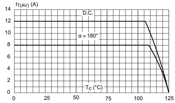
**Figure 3. Average and DC on-state current versus ambient temperature (DPAK, D<sup>2</sup>PAK)**
