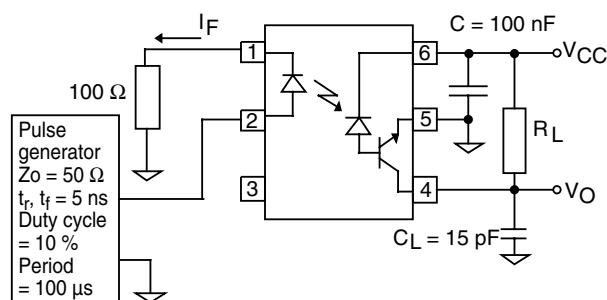
Fig. 1 - Test Setup
