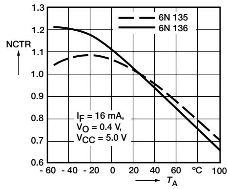
Fig. 10 - Current Transfer Ratio (Normalized) vs. Ambient Temperature
