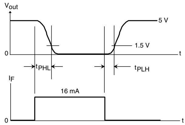
Fig. 2 - Switching Time Measurement
