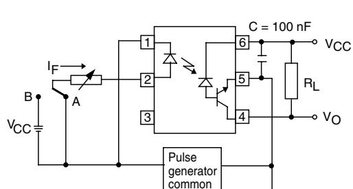
Fig. 3 - Common Mode Transient Test
