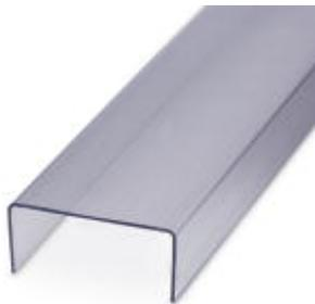
U profile cover, for covering terminal strips, internal dimensions: 100 x 40 mm, 2 mm thick, produced according to length specifications, additionally required: 2 E/UK end brackets or E/U end clips and 2 VAH cover brackets, maximum supply length: 2 m
