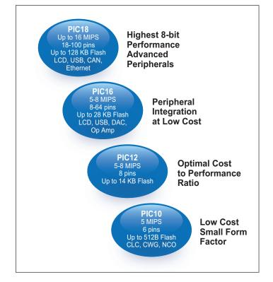
There are hundreds of 8-bit PIC microcontrollers to choose from ranging from 6 to 100 pins and up to 128 KB Flash that are pin and code compatible across the portfolio. PIC microcontrollers with XLP technology feature the world's lowest active and sleep power consumption with flexible power modes and wake-up sources. MPLAB® Integrated Development Environment supports all PIC microcontrollers with C Compiler support and common development boards.
