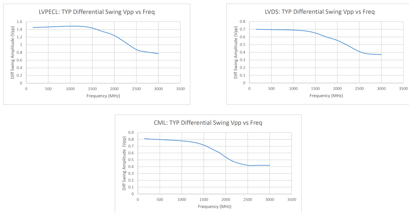
Figure 2.1. Typical Clock Output Swing Amplitudes vs. Frequency
