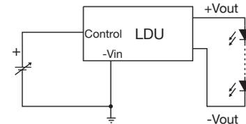
A Control Voltage lower than 0.15 V will turn the output off
