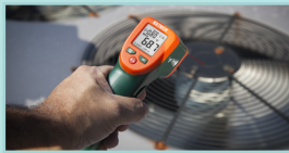
Test for temperature in HVAC systems
