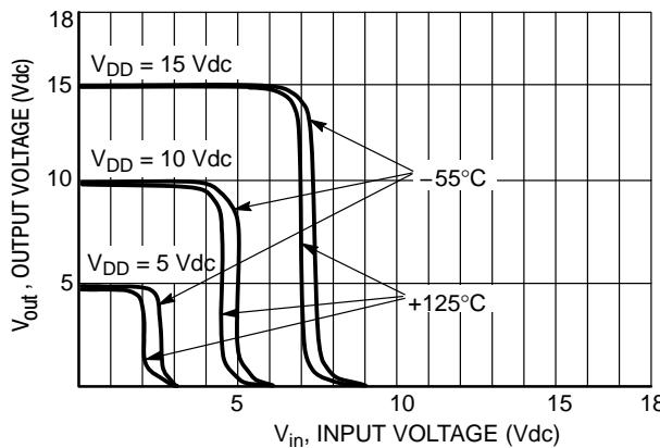
Figure 4. Typical Voltage Transfer Characteristics versus Temperature
