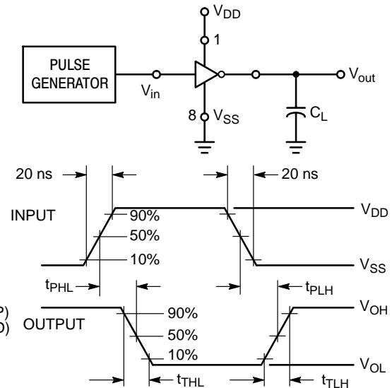
**Figure 8. Switching Time Test Circuit and Waveforms**
